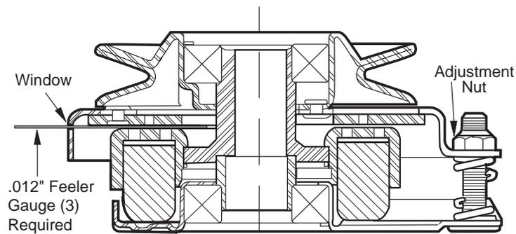
Inserting the Feeler Gauges
