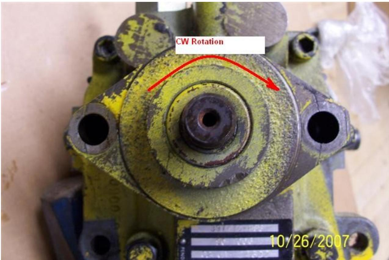
When the input shaft is now driven CW, the suction again comes from the bottom and pulls oil up from the sump in the rear axle, through the filter, through the charge pump, and off to the main hydro pump. If you were to just turn the charge pump around without changing the input rotation it would be trying to draw oil from the main pump instead of the sump and again nothing would work.
