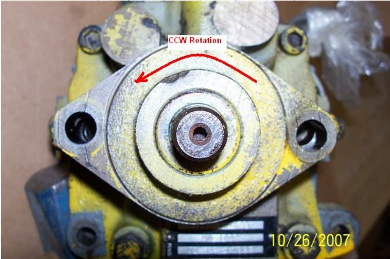
The secret to the reversing is that the inside of the housing is machined off-center so that the driven gerotor part of the charge pump is offset to the right as you are looking at this.
