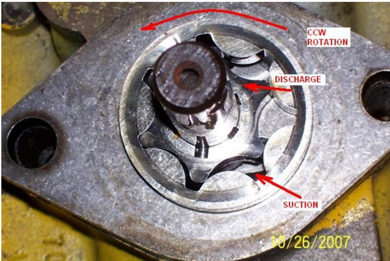
So then, when the charge pump turns CCW, the gear rotates CCW and pulls oil up from the sump in the rear axle, through the filter, through the charge pump, and off to the main hydro pump. If you were to just turn the motor around and change the input rotation it would be trying to draw oil from the main pump instead of the sump and nothing would work.
