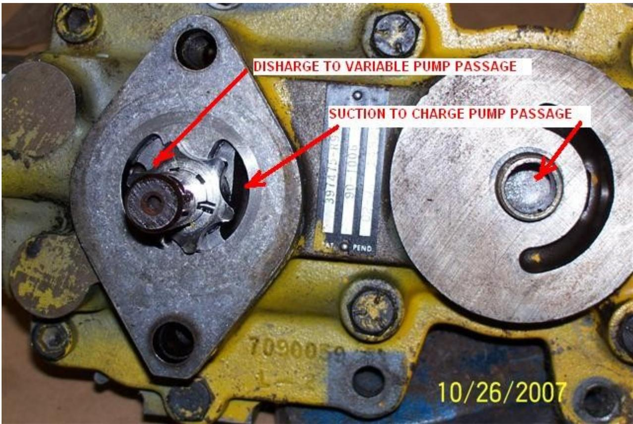
Now when you change the flat side of the charge pump housing to the right side, the off center machining on the inside places the driven gerotor to the left side of the driving gear.
