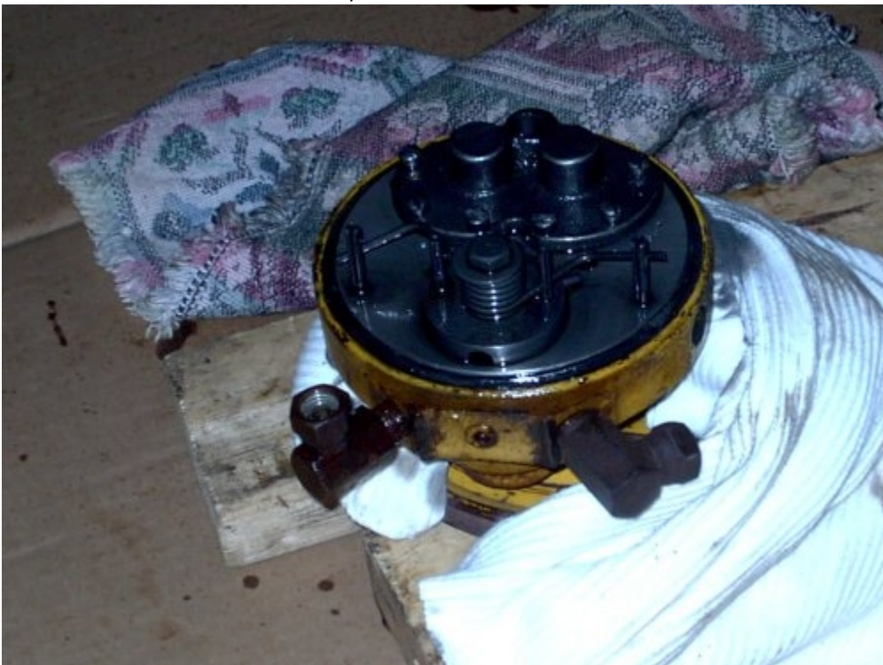
this is what the pump will look like when the reservoir is off showing the center return spring on the reservoir side of the spool, and the pump, which is built into the casting with the gear cover with six screws holding it on.
