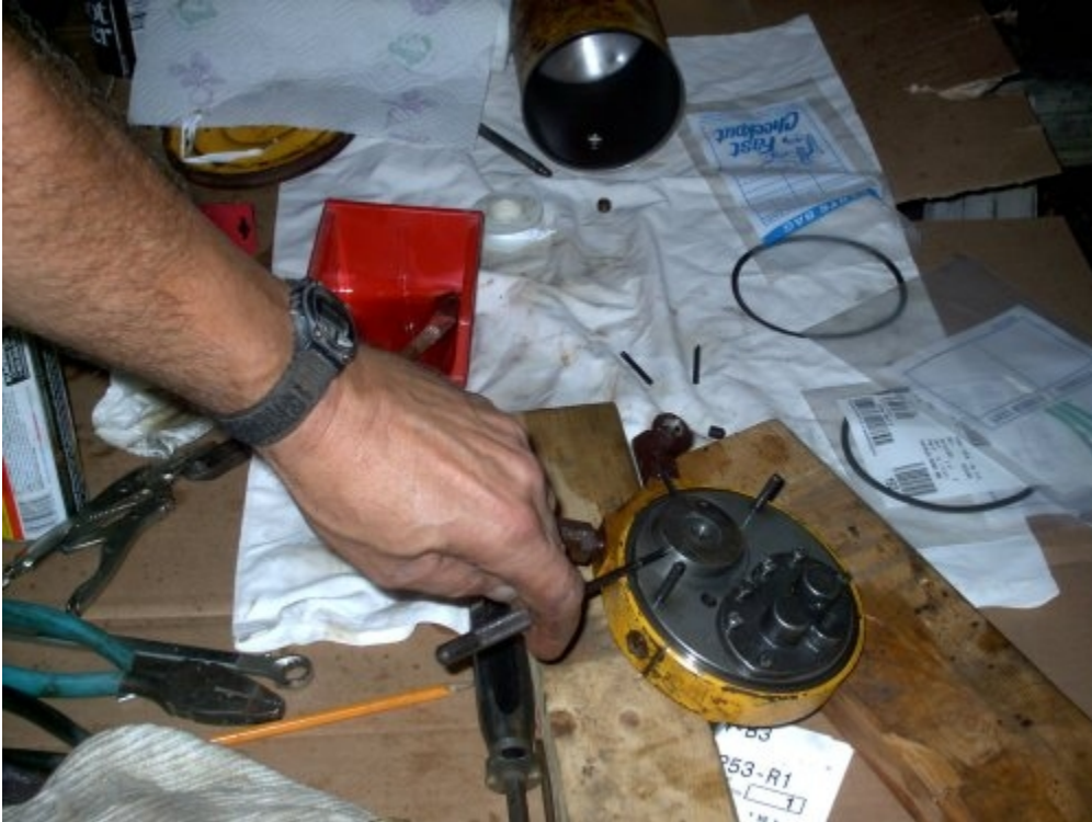
the roll pin retainers in place
