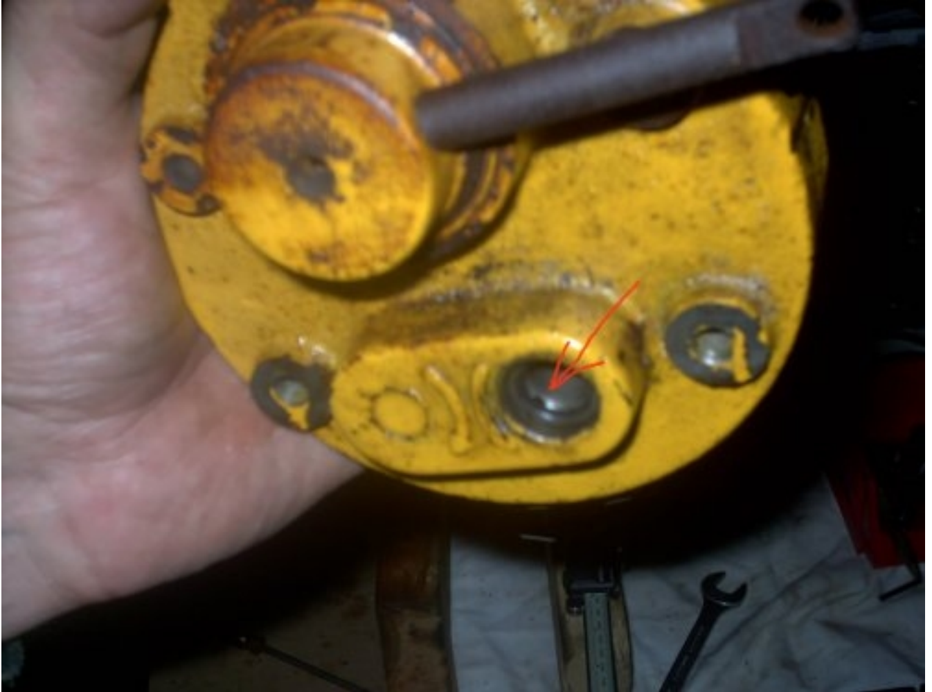
first seal installed showing drain hole still open
