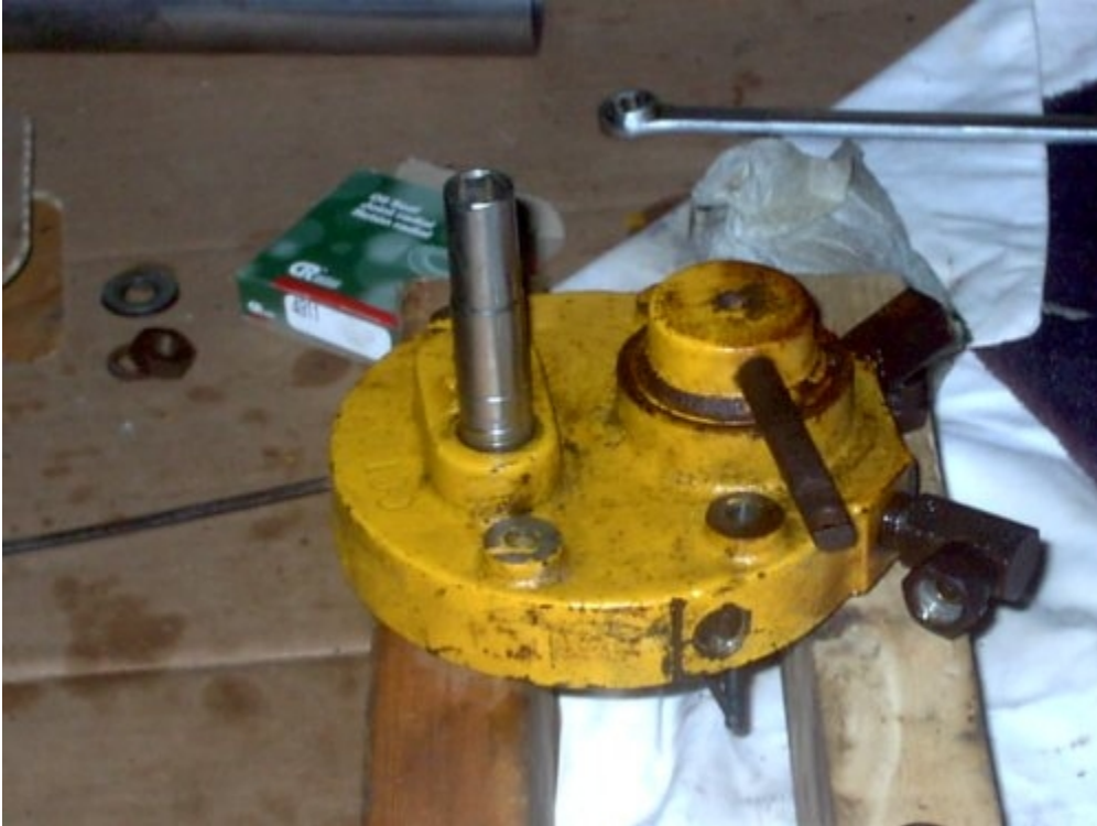
found a socket the right size to drive in first seal
