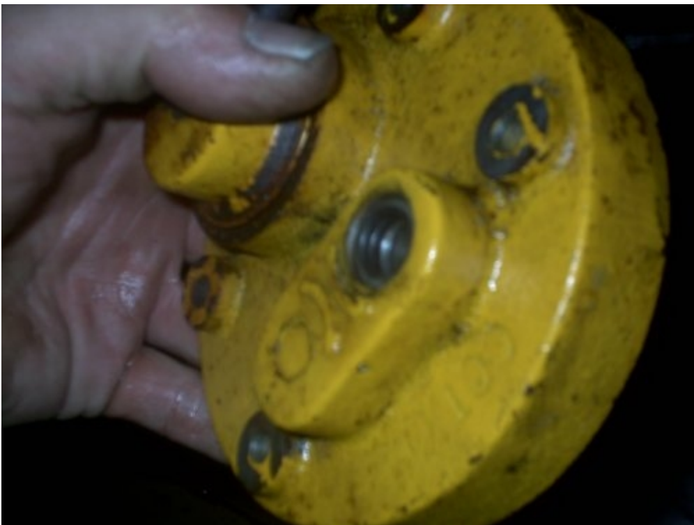
both seals in and drain hole still showing, but not in this picture! slight space between the seals to let individual seal lips move independantly
