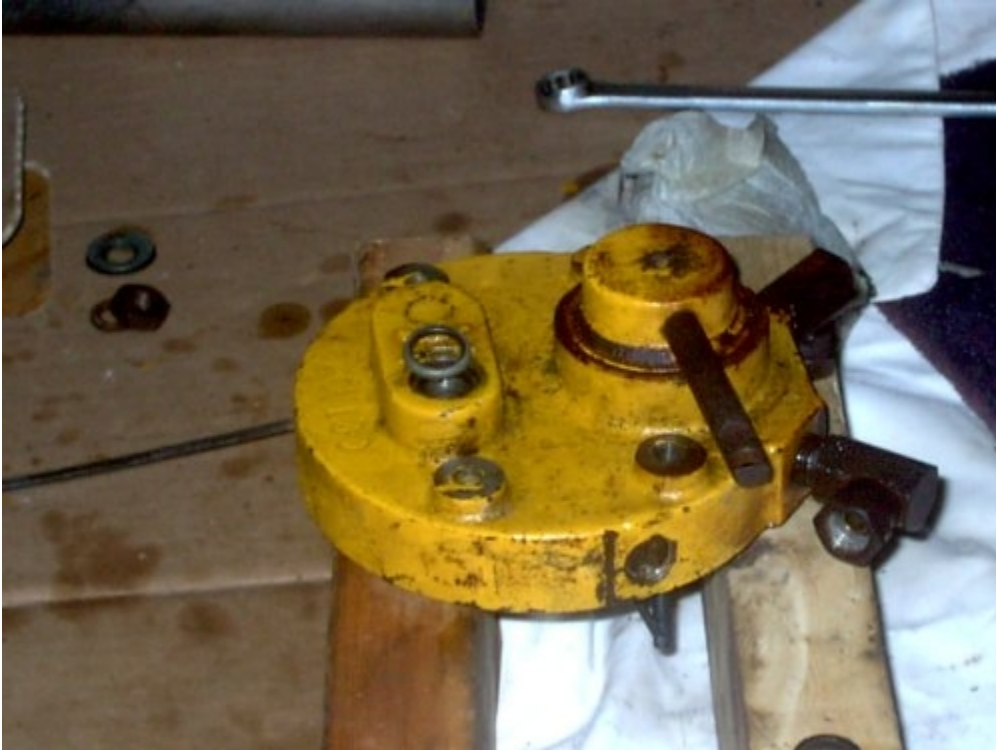
second seal goes in next, slightly below surface of casting, hole is chamfered
